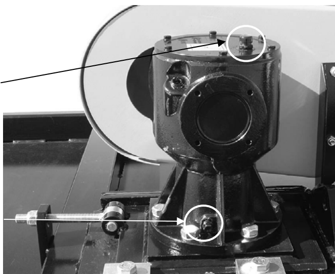
Breather-/oil fill-nipple with dipstick
