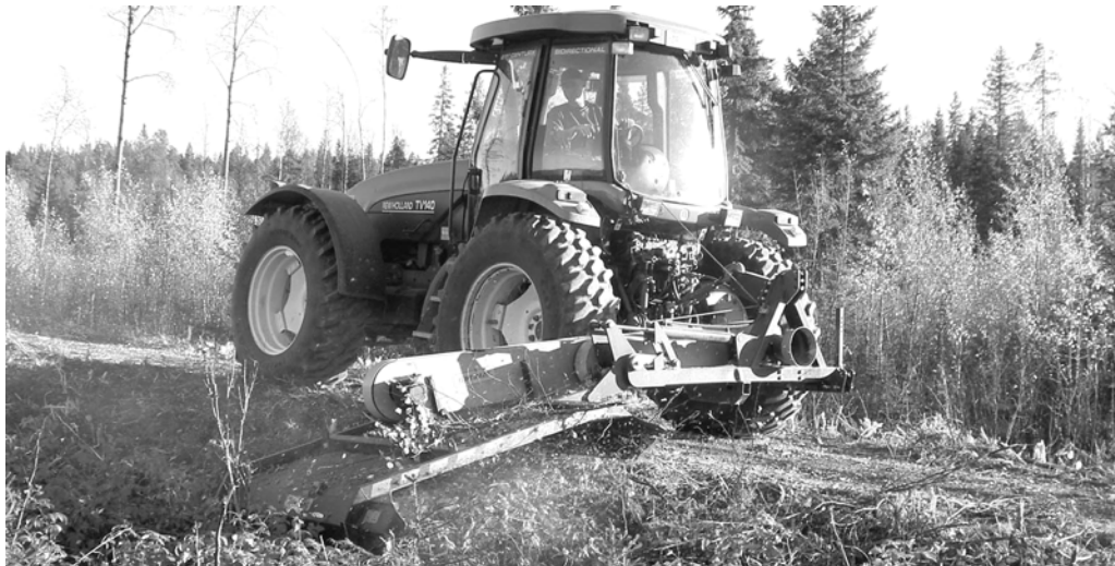
M-160, Mounted at the rear of a reverse drive tractor.
