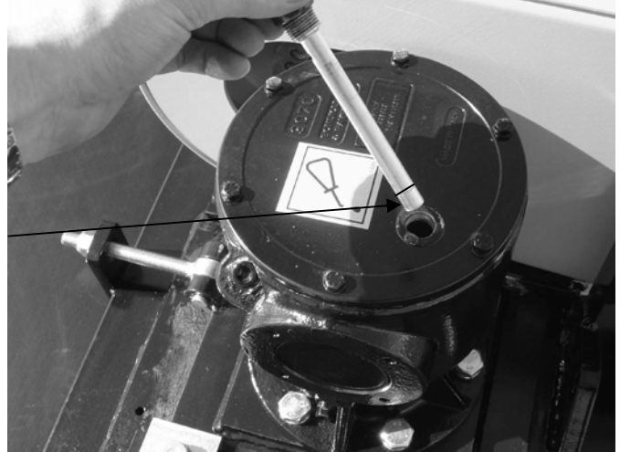
Breather-/oil fill-nipple with dipstick
